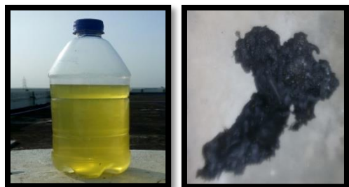
Fig. 3. Sample of crude Plastic fuel collected and solid black residue
